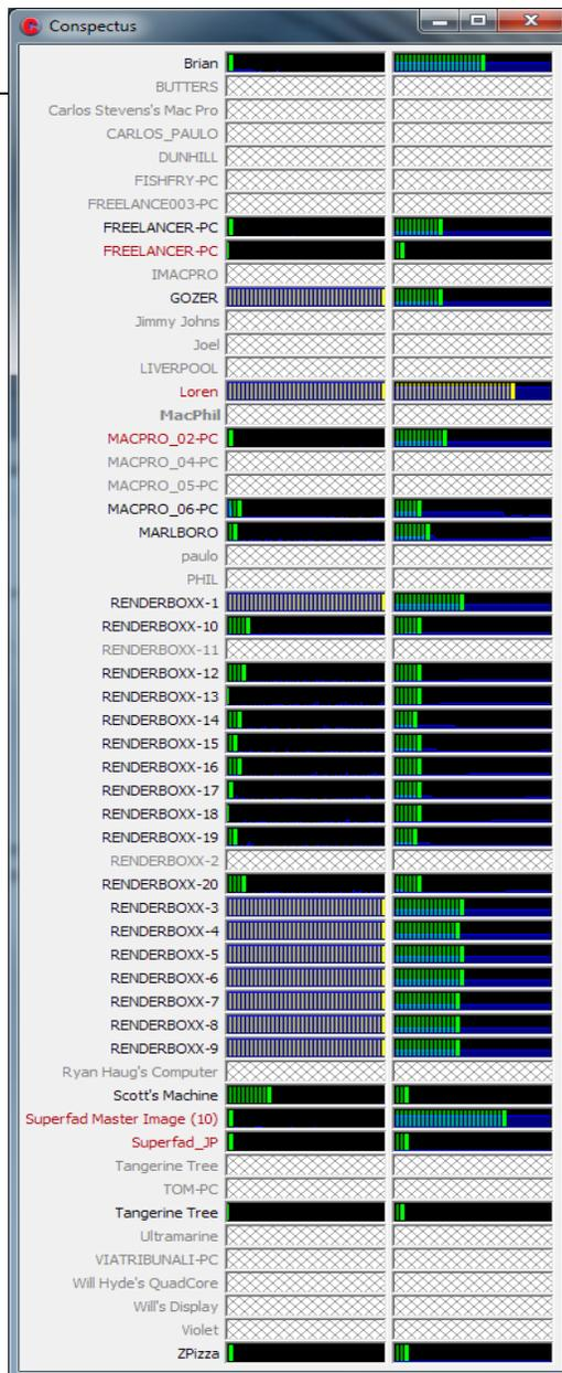
Conspectus is a simple graphical view of the name, CPU status and memory status of every Engine in the system. It does not provide any control for the Engines.
